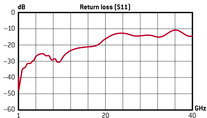
Typical responses of S11 and S21 Measurements on a PTFE 50 Ohm substrate
