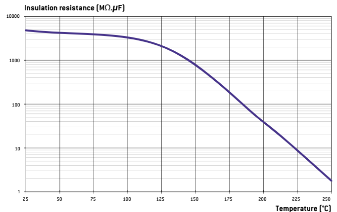
X7R: TYPICAL INSULATION RESISTANCE VERSUS TEMPERATURE
