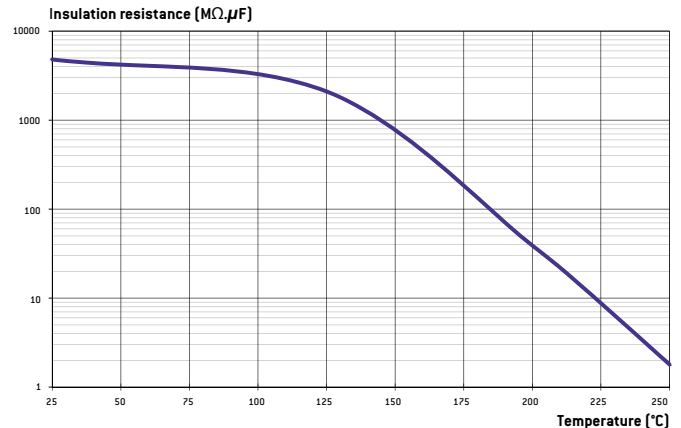
X7R: TYPICAL INSULATION RESISTANCE VERSUS TEMPERATURE
