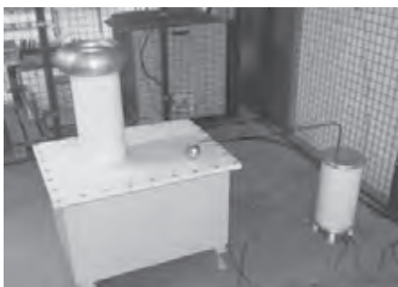
Partial discharge equipment available up to 100kV
