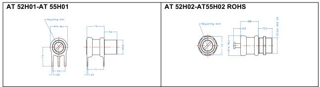
Terminal with two legs is in contact with tuning rotor
